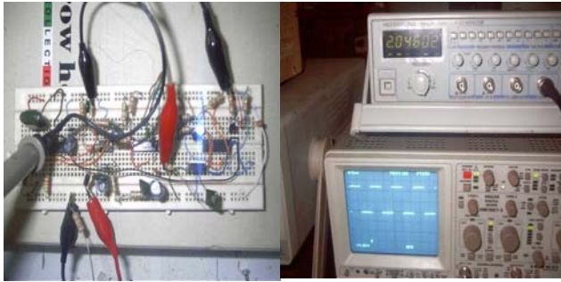
Fig. 14 PLL CD4046 of VCO output waveform
